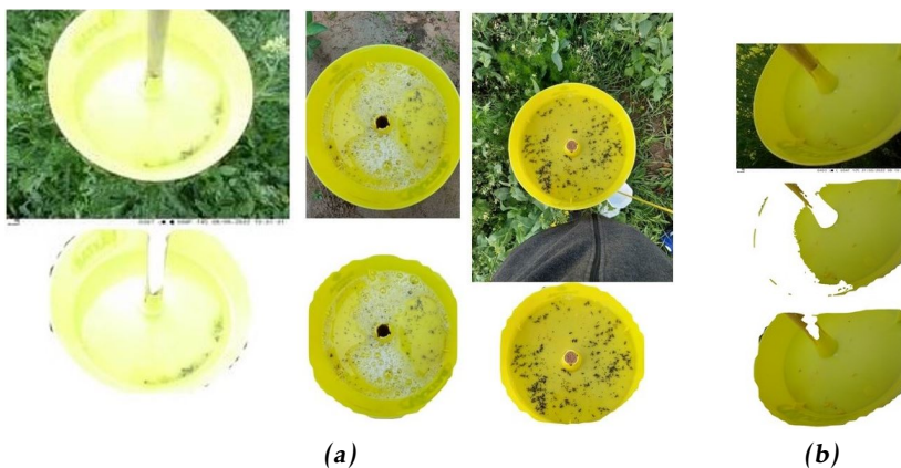
Figure A.2: Mask R-CNN background removal on cup traps. Two of the images were cropped to detection. The a) are examples of passing results. The H3G image in b) needed a rerun.
